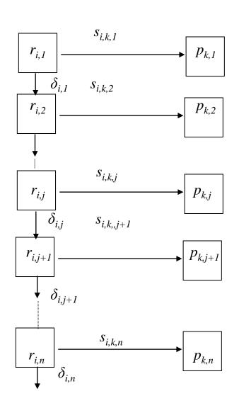
Assume now that we do the same cascade for each hot stream, while we do not cascade the cold streams at all. In addition we consider heat transfer from hot to cold streams in each interval.
