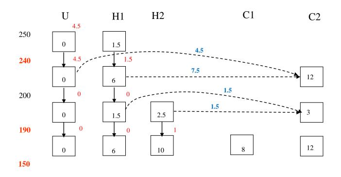
We finish in interval 4 using H1 first with C1, then H2-C1 followed by H2-C2 and then U, which is now been augmented
