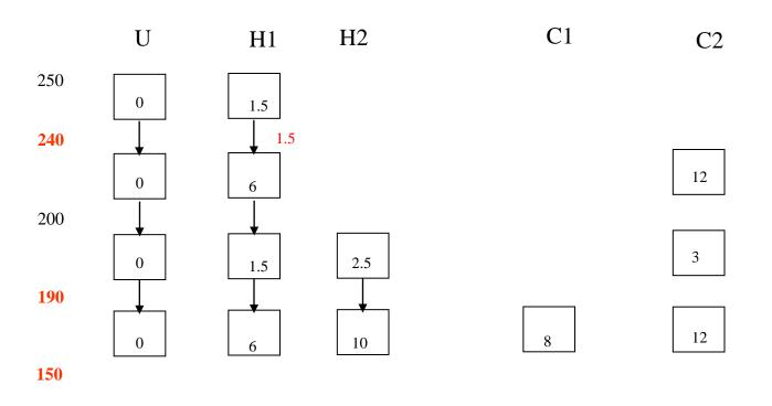
We now send 7.5 to the cold stream and use utility cascaded to fulfill the 12 units the cold stream C2 requires
