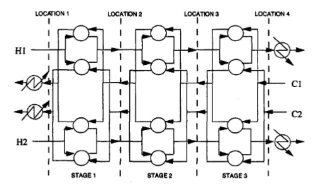
At each stage every hot/cold stream splits and matches with all other (cold/hot) stream. H1 and C1 are highlighted
